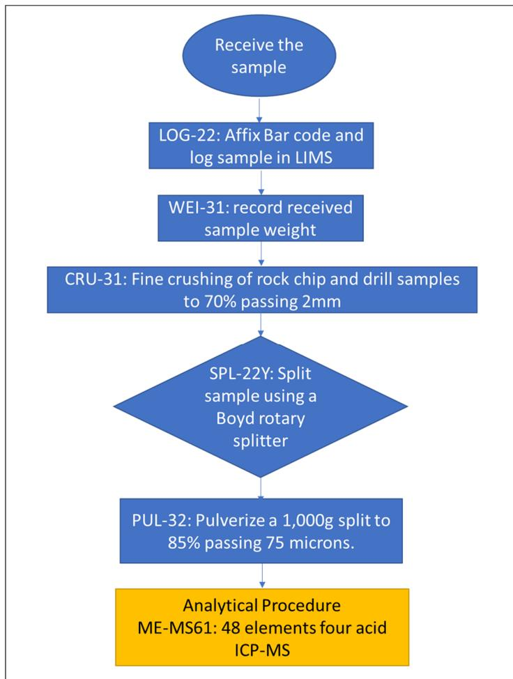
Figure 11-2 ALS Global sample preparation flowchart and analytical method (Corcel Minerals, 2022).
